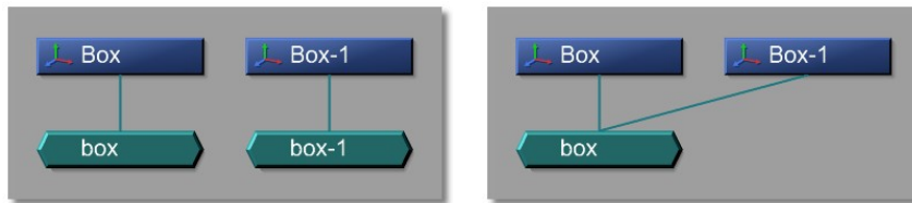
Figure 2.2. Schematics view of a duplicated (left) versus instanced (right) Object
